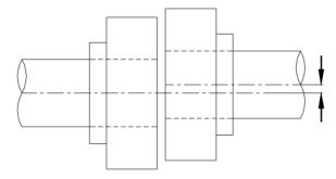
d3-By fitting couplings be sure that the two shafts are not angular miss-aligned.
