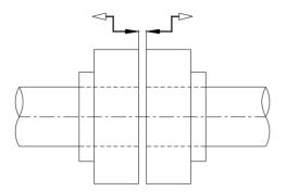
d2-By fitting couplings be sure that there is no exantricity between the two shafts.
